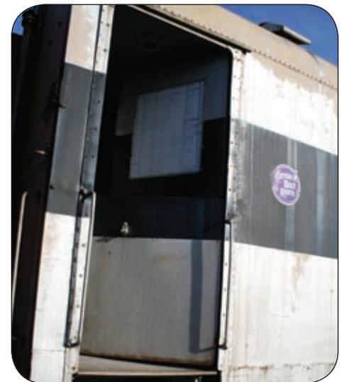
*Fabricated doors currently installed on Coach 1318. These will be replaced by authentic Pullman doors.*
