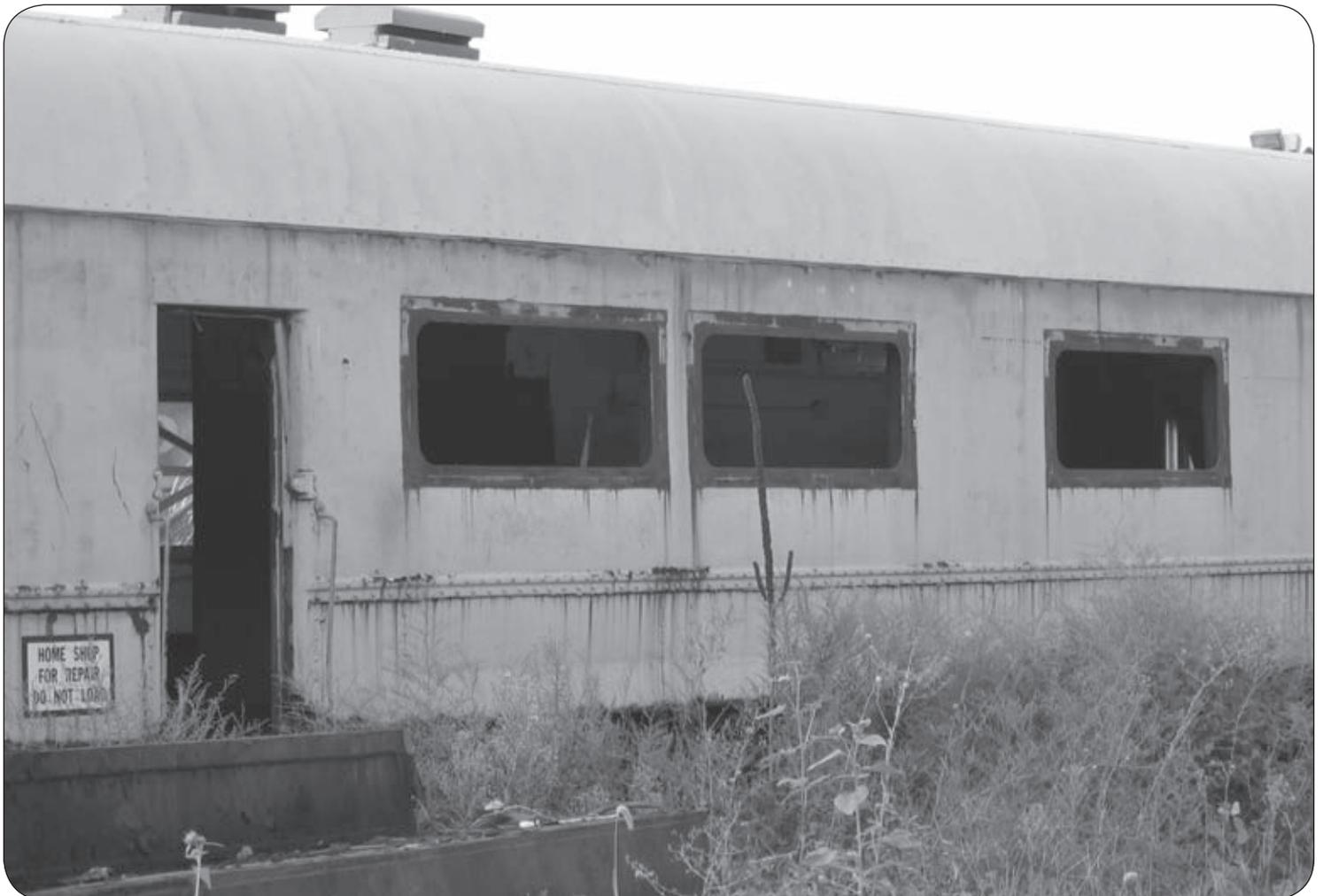
This is the kitchen end of 741. You can see from this photo the new sheet metal for the roof and the new kitchen vents. The light-colored material on the roof is the rubber sealer. Note the original Erie Lackawanna paint is visible around the kitchen windows. (Photo by Michael Steinberg)
