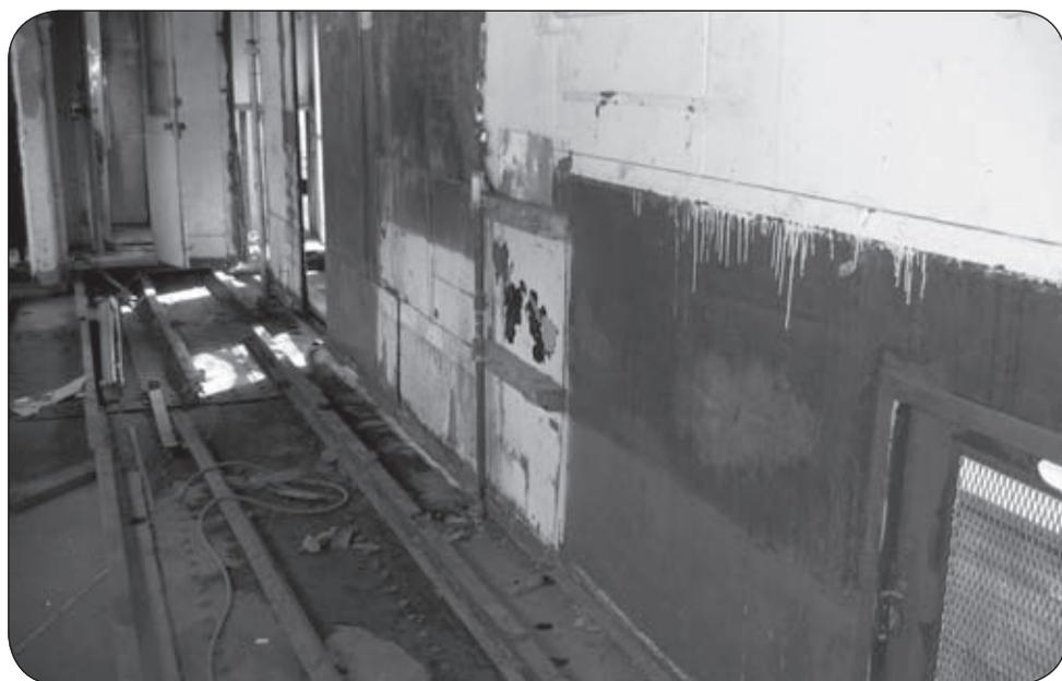
*The wall separating the kitchen and hallway of Diner 741. Notice the doorway cut into the wall to access the hallway. This wall will be replaced by Midwest Locomotive. (Photo by Becca Steinberg)*
