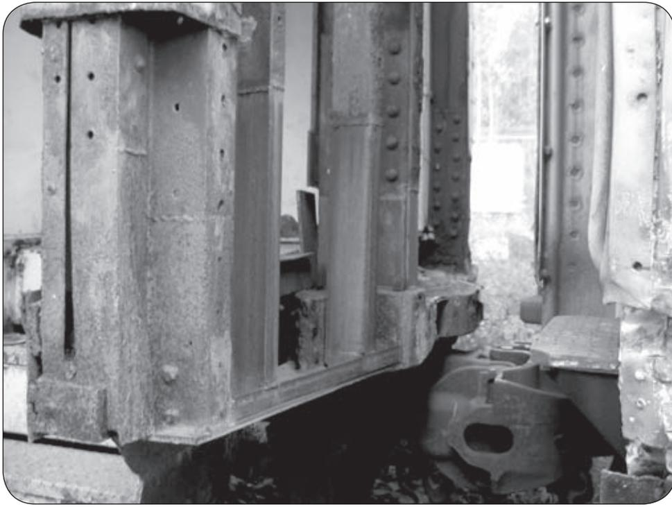
New I-beam supports and a new crash post I-beam to the left have been welded in place. New sheet metal will eventually cover this section. (Photo by Michael Steinberg)
