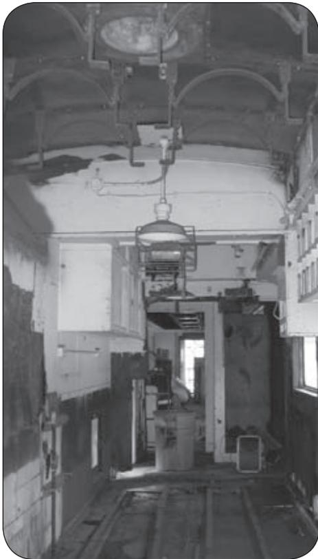
Looking towards the dining area of 741. You can see the new roof and the supports for the fresh water tanks above. The original kitchen cupboards will be retained in their original locations. Note the kitchen light fixtures. (Photo by Becca Steinberg)
