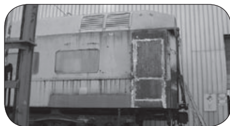
Diner 741 after MoW doorway has been sealed. (Photo by Midwest Locomotive)
